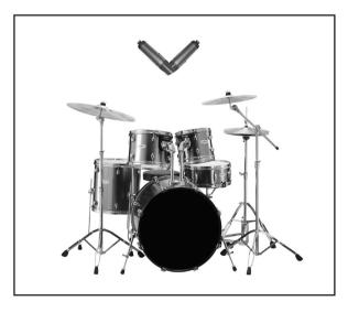
In this diagram, two WA-87's are used in a coincident pair, also known as XY configuration, to record stereo drum overheads.
